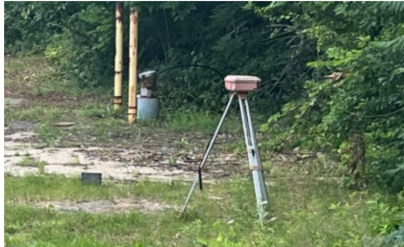
An example of an air monitoring station
